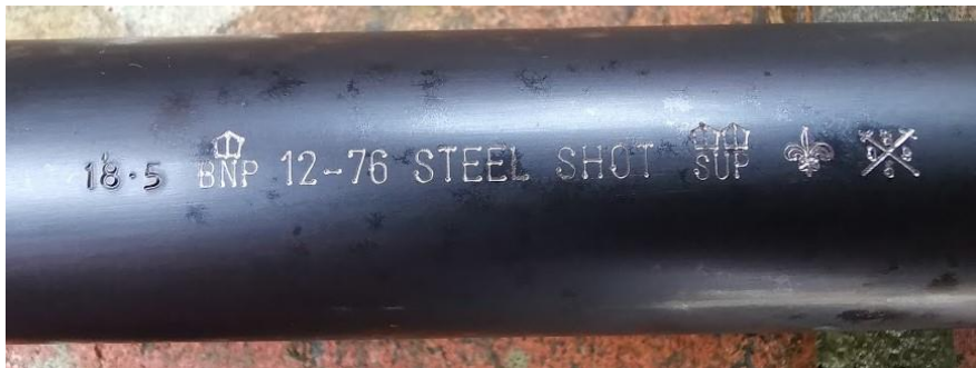
A modern gun showing nitro, superior and steel proof for 76mm (3 in) cartridge. The 'fleur-de-lis' shows it is suitable for high performance steel cartridges.
